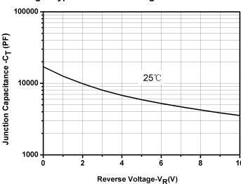
Fig.3-Capacitance vs. Reverse Voltage
